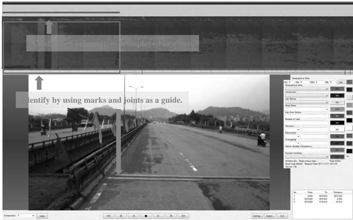
Figure 10.17 Example of Identify Position for a Bridge
