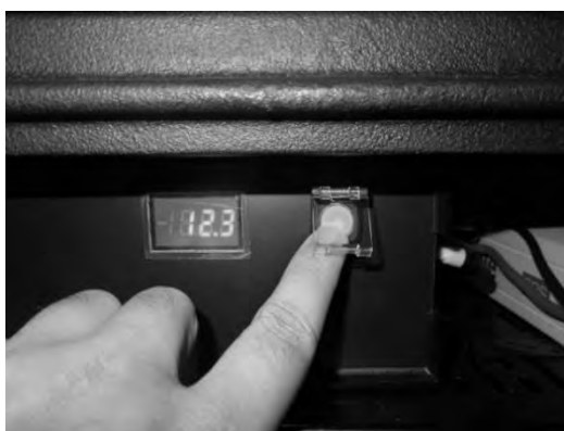
Figure 6.33 Shutting Down the System
