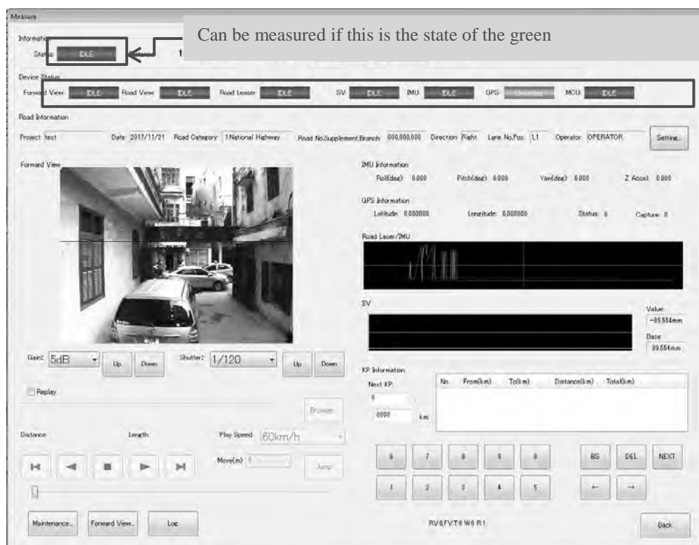
Figure 6.15 Operation State (Green)
