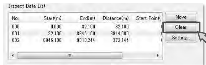
Figure 9.31 Deleting a Section
