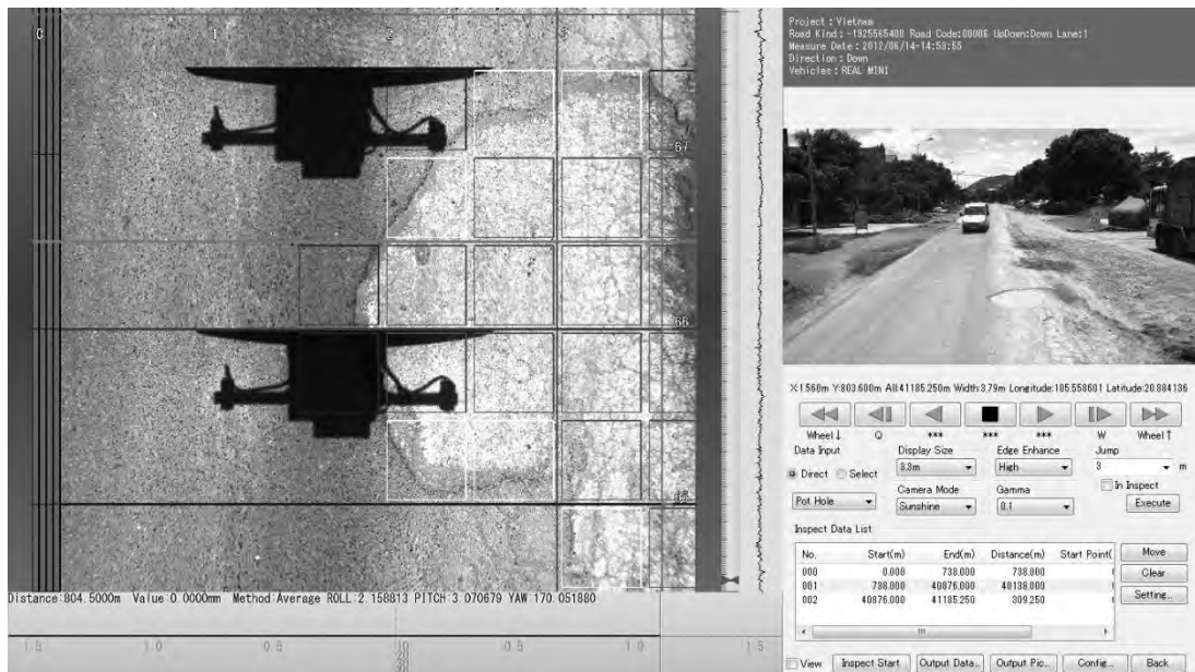
Figure 9.50 Example of Crack Recording Operation
