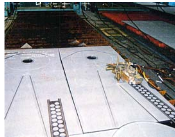
GAS Frame Cut
