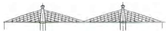
Hatley pointed out that in-plane flexural rigidity of Harp type is inferior to that of Radial type
