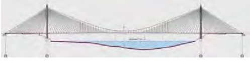
Combined [earth and self-anchored cable-stayed] bridge and [suspension] bridge 3 rd Bosphorus Strait Br. (Istanbul in Turkey)
