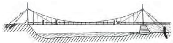
The bridge was collapsed in 1817 , a half year after opening The reason is chain broken due to wind-induced vibration
