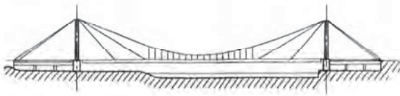
Proposal for a railway bridge with a span of 750-m over the Elbe river near Hamburg, Germany
