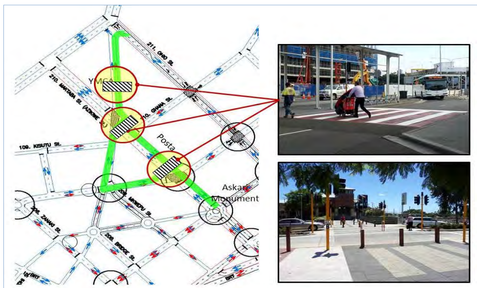
Figure C9: Location & design of raised crossings
