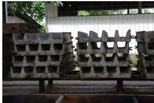
Figure 5.3.25 Molds of PC sleeper (4 PC sleepers can be produced by one mold )
