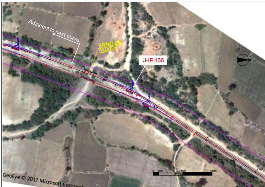
Figure 5.2.9 Curve Improvement of U-IP.136
