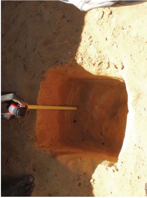
Figure 15. Pre-soaking the hole
