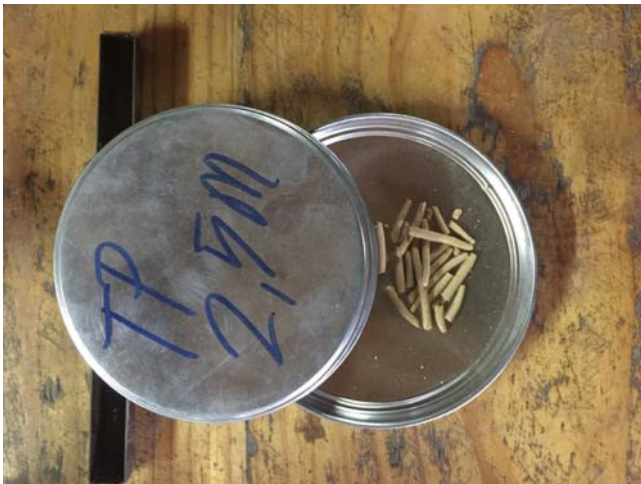
Figure 22. Plastic soil at 2.5m
