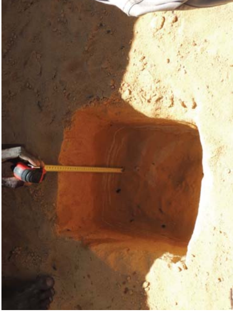
Figure 15. Pre-soaking the hole
