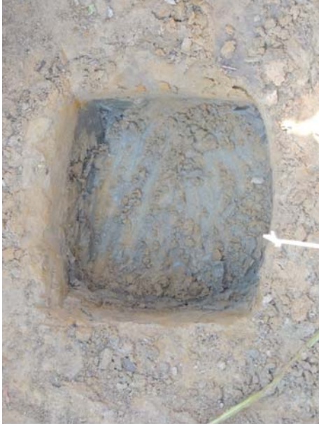
Figure 13. Detail of permeability test hole
