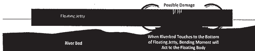
Fig. 3. Image of Damage to the Floating Jetty due to Siltation
