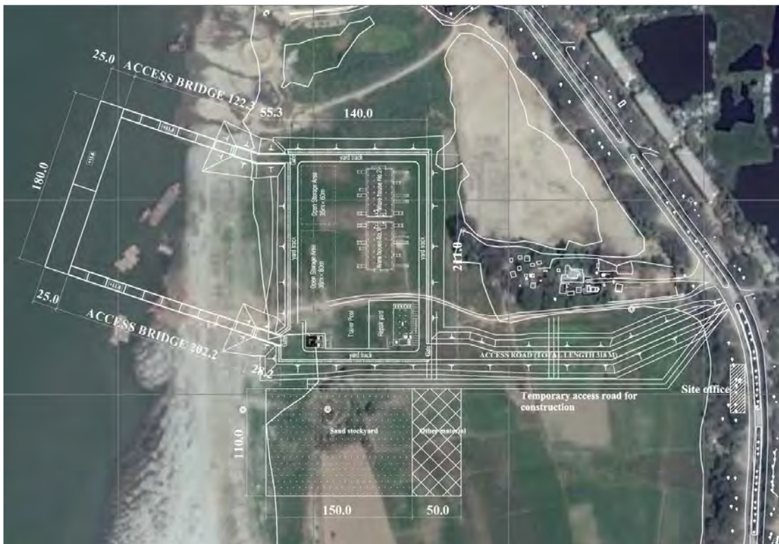
Figure 1-2-34 Layout Plan of Option (b): building and using only a new road
