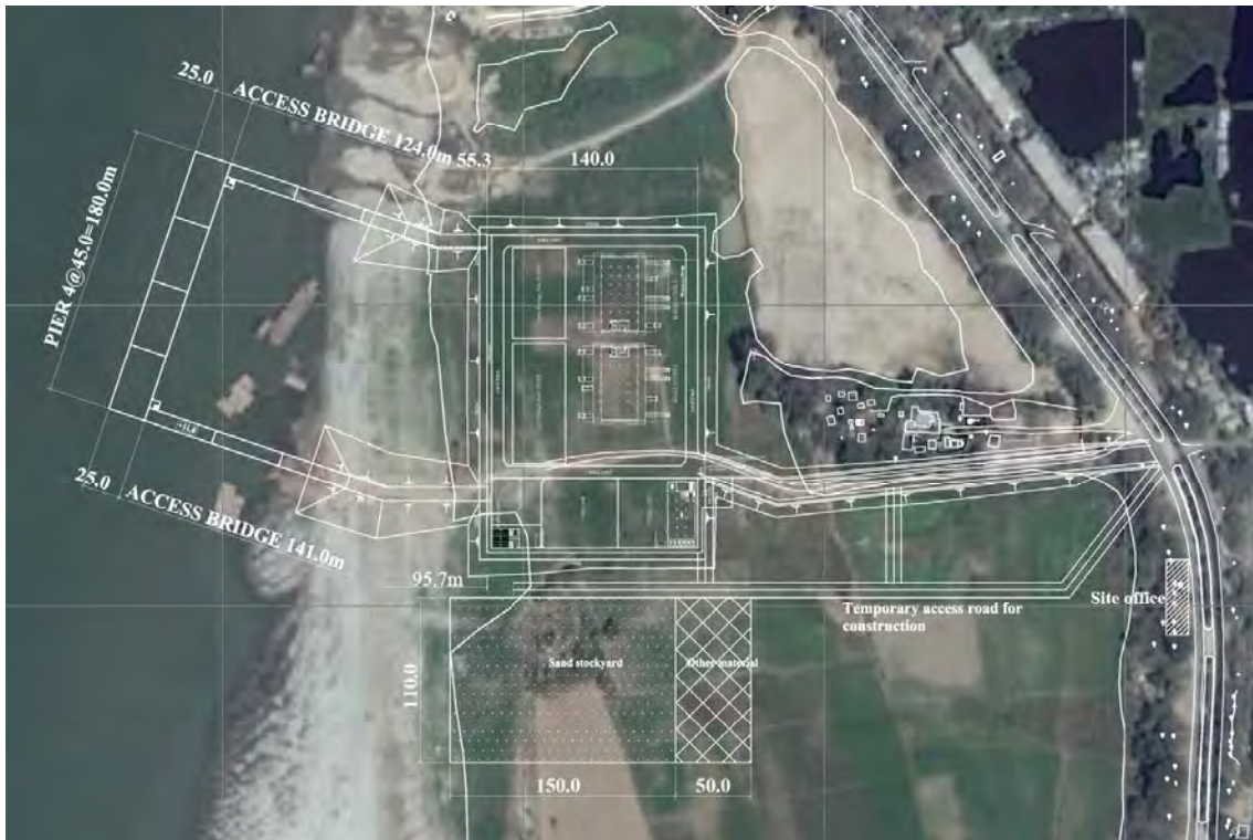
Figure 1-2-33 Layout Plan of Option (a): using existing road and new road
