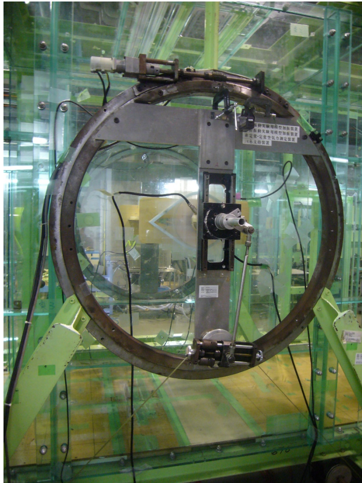
Fig.5.4.3 Experimental setup for forced vibration test
