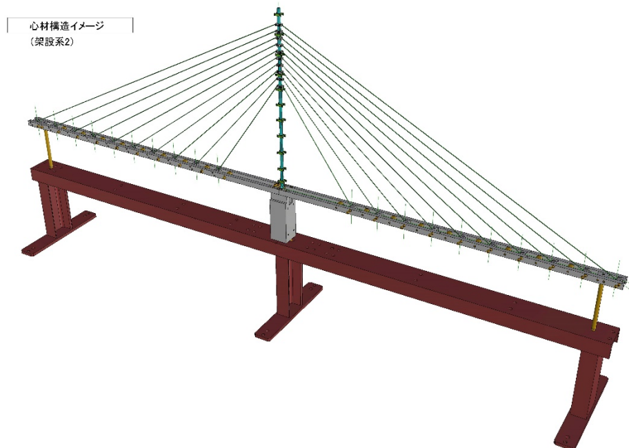
Fig.2.2.10 3-D image of elastic bar for the tower and rigid bar for the main girder (The supports at both ends of the model are to keep the girder as rigid.)
