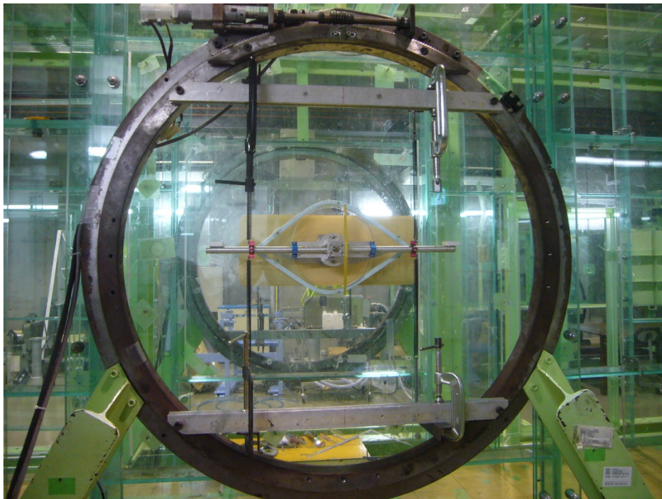
Fig.5.4.1 setup of the free vibration test of the section model
