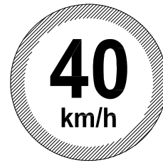
TS-3 SPEED LIMIT 40 KM/H SIZE: 600 MM DIAMETER
