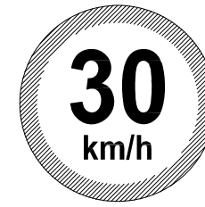
TS-4 SPEED LIMIT 30 KM/H SIZE: 600 MM DIAMETER
