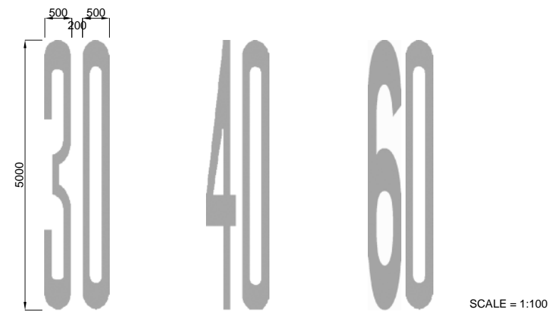
PM-1 SPEED LIMIT 30 KM/H PM-2 SPEED LIMIT 40 KM/H PM-3 SPEED LIMIT 60 KM/H
