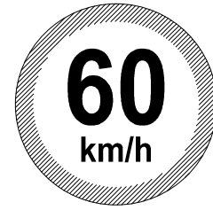
TS-2 SPEED LIMIT 60 KM/H SIZE: 600 MM DIAMETER
