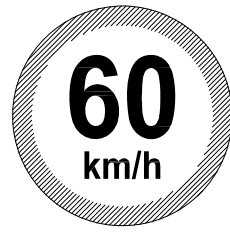
TS-2 SPEED LIMIT 60 KM/H SIZE: 600 MM DIAMETER
