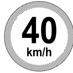
TS-3 SPEED LIMIT 40 KM/H SIZE: 600 MM DIAMETER
