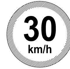
TS-4 SPEED LIMIT 30 KM/H SIZE: 600 MM DIAMETER
