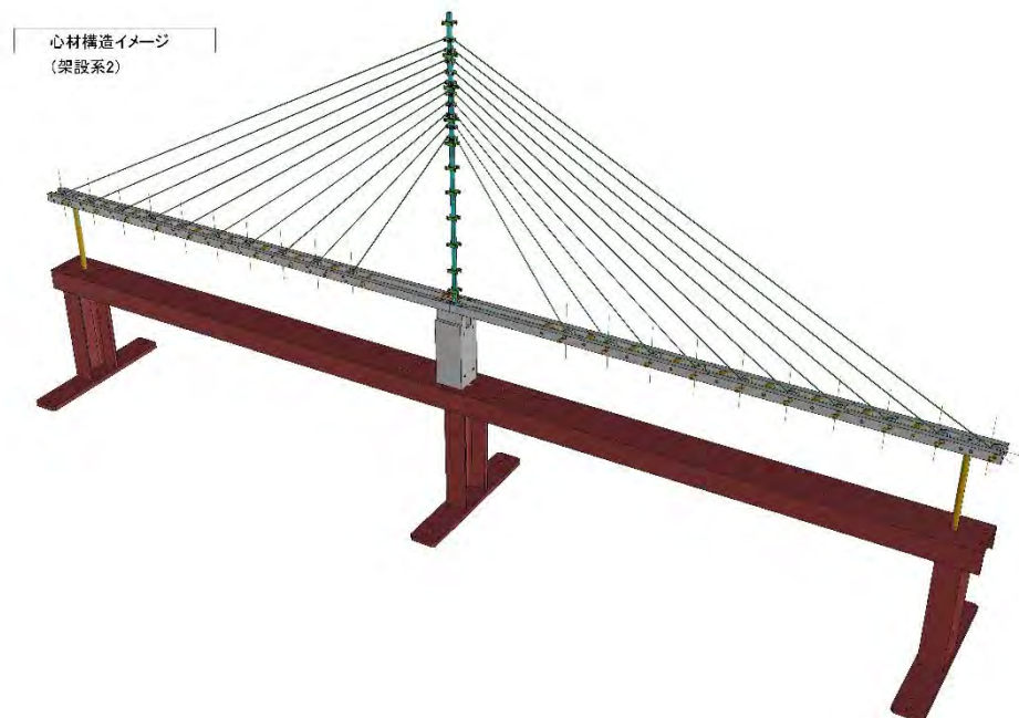
Figure 4.2.258 3-D image of elastic bar for the tower and rigid bar for the main girder (The supports at both ends of the model are to keep the girder as rigid.)
