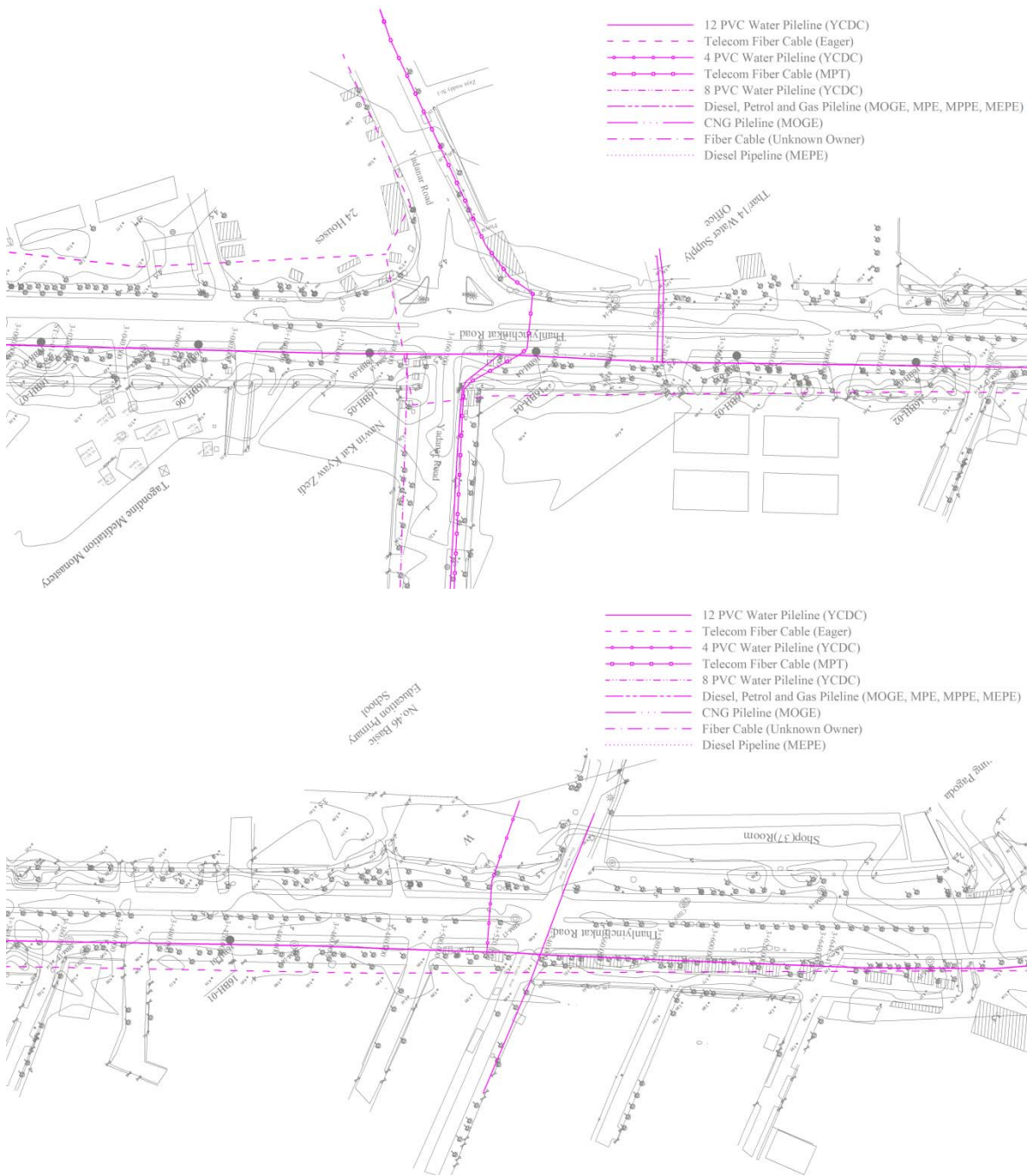
Figure 2.5.1 Existing Underground Utilities Layout
