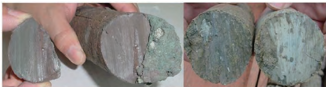
Figure 2.3.8 Example of Slip Surface on Tuff Core that had a Clear Slickenside 30
