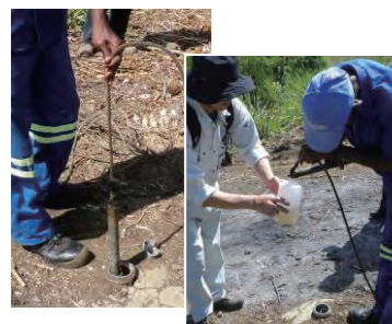
The borehole sample is collected using a water trap (bailer), and immediately transferred to polyethylene bottles.
