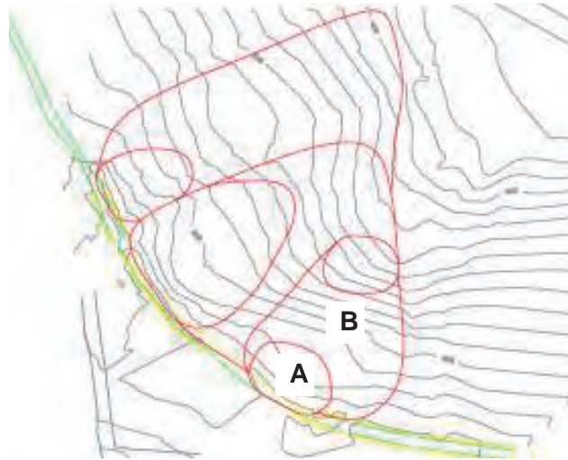
Figure 6.2.13 Example Case that Minor Landslides exist within a Large Landslide Area. If the soil removal work is adopted at head part of landslide A, it will affect the stability of landslide B (source: JET)
