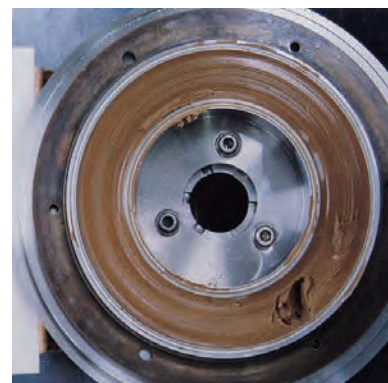
Figure 2.1.22 Schematic Diagram of Sample for Ring Shear Test 17
