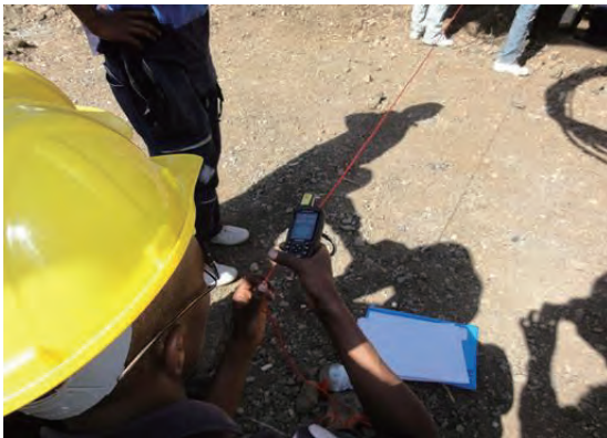
Photo A-1 Positioning of drilling points by GPS (Source: JET)
