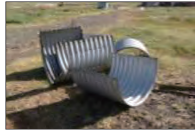
Photo 7.2.1 Corrugated Steel Half-Pipe (source: JET)
