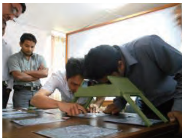
Figure 2.1.2 Aerial Photo Interpretation using a Stereo Scope (source: JET)
