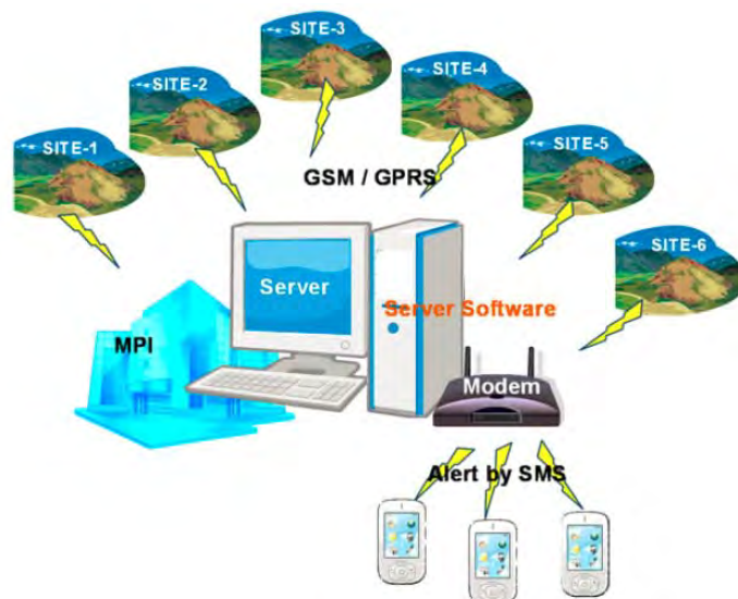
Figure 2 Image of the remote monitoring system (Source: JET)
