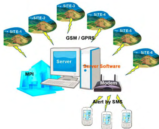
Figure 3.3.2 Image of the remote monitoring system (Source: JET)
