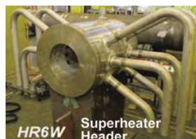
Superheater header mock-up
