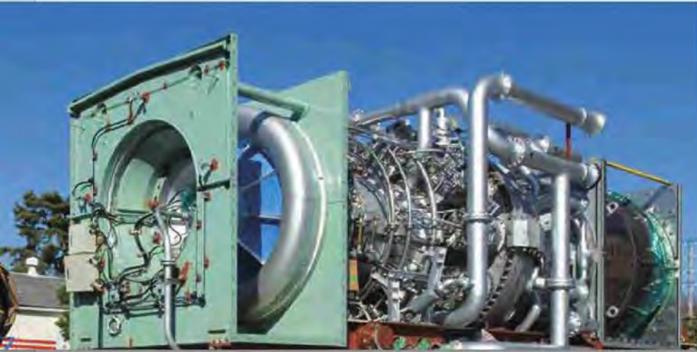
H-100 Gas Turbine on Trailer
