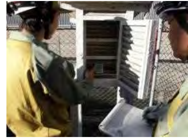
Recording temperature and humidity (Outside)
