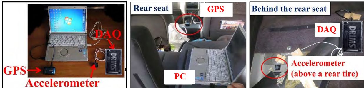
Figure-4 Typical Installation of DRIMS Equipment into Vehicles
