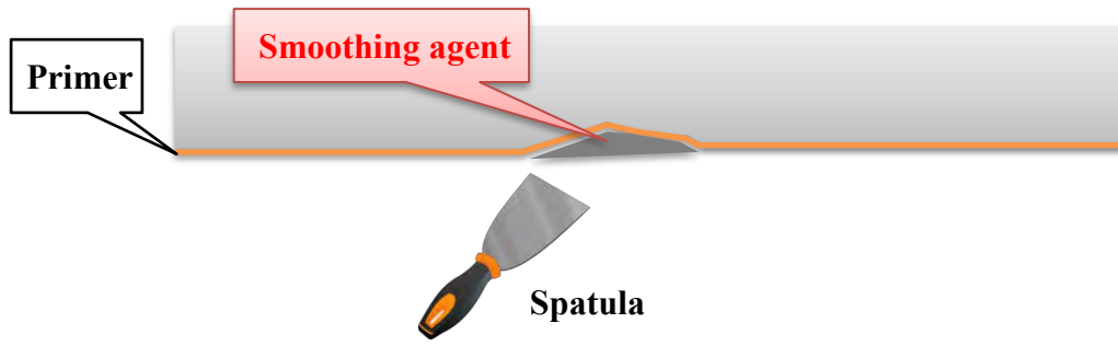
Fig. 5.2.2.11 Applying smoothing agent
