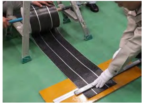
Photo 5.2.2.3 CFC (Carbon Fiber Cloth)
