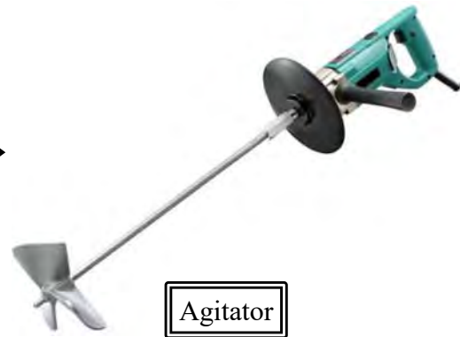
Photo 5.2.2.27 Mixing material (Impregnating resin)
