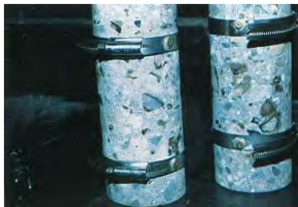
Photo 5.2.12.5 Sampled cores banded for change of perimeter measurement
