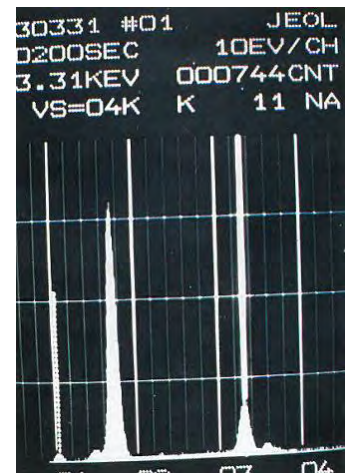
(c) X-ray intensity spectrum by elements exuded gel
