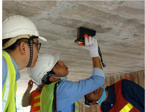
Photo 5.2.2.10 To measure moisture of the concrete surface
