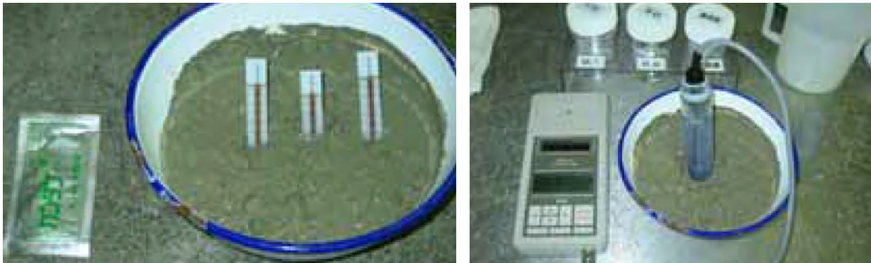
Photo 4.5.6 Chloride Ion Content Test
