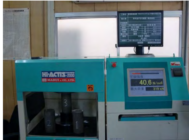
Photo 4.5.3 Compressive strength test machine
