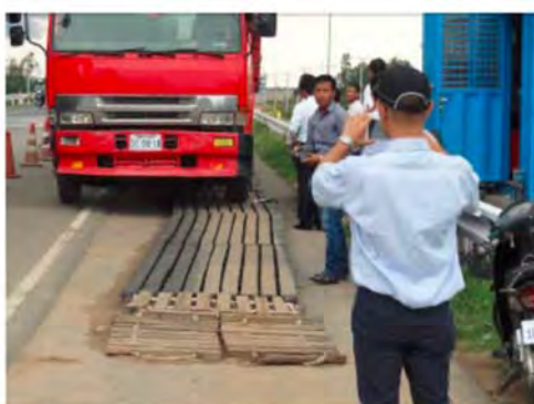
Not enough space and imbalance ground elevation for load measurement
