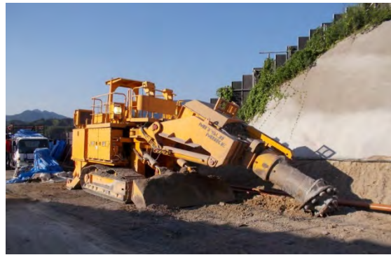
Figure 3-26 Drilling and Blasting (top-left), Mechanical Excavation by Boom Header (top-right) and Mechanical Excavation by TBM (bottom-left)
