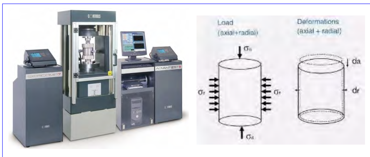
Figure 5 An Example of Stress Path Triaxial and Uniaxial Compression Test System
