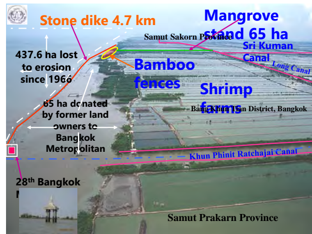
Figure 2.9.4: Mangrove reforestation by local knowledge with Bamboo Fences
