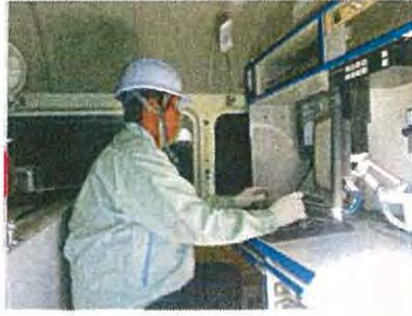
Pipe O&M Trainig (TV camera survey)
