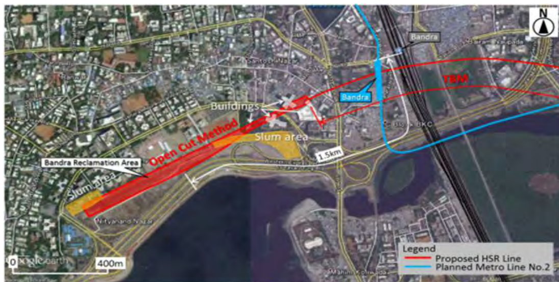
Figure 8.1.5-9 Setting HSR Station Underground after Removing Expressway Seaside (Plan A)
