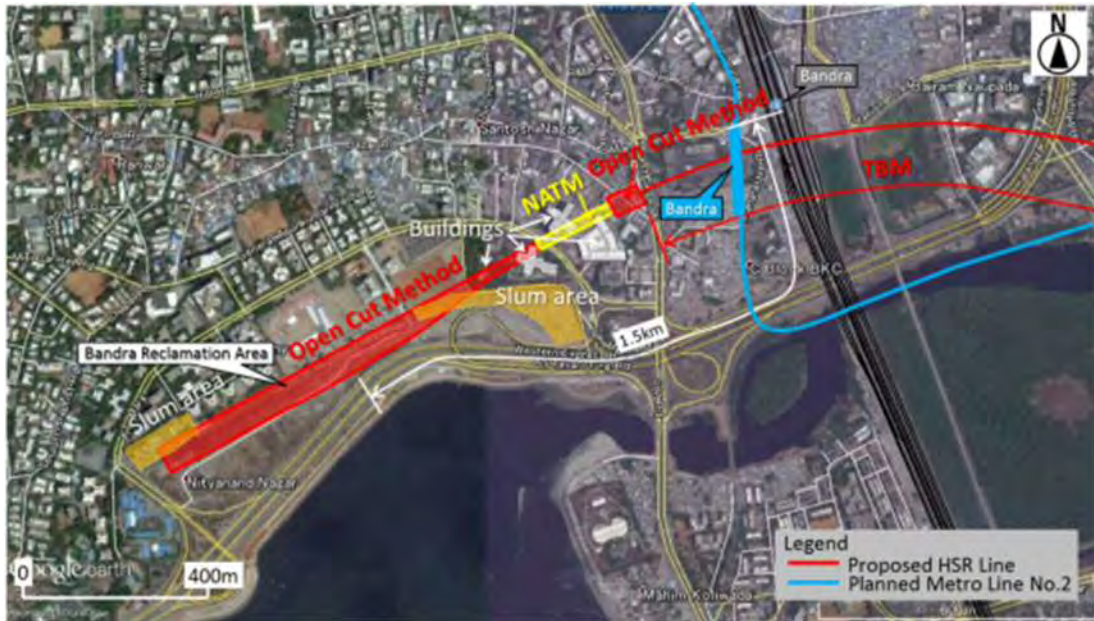
Figure 8.1.5-11 Setting HSR Station Deep Underground to Passing under Buildings (Plan C)
