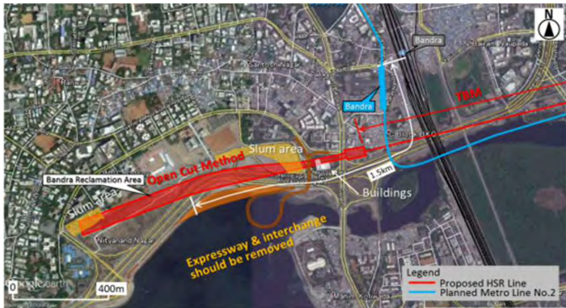
Figure 8.1.5-9 Setting HSR Station Underground after Removing Expressway Seaside (Plan A)
