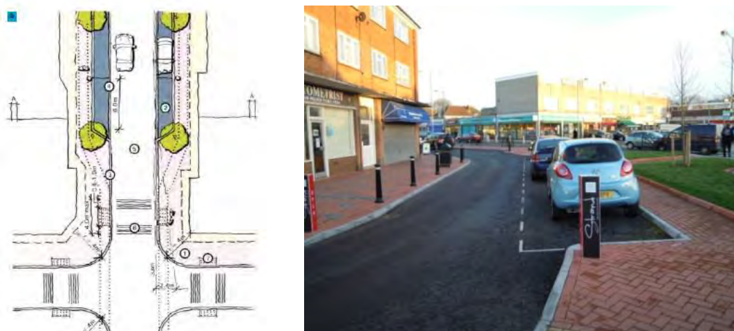
Figure 7.8-11 Design of On-street Parking and Picture of On-street Facility
