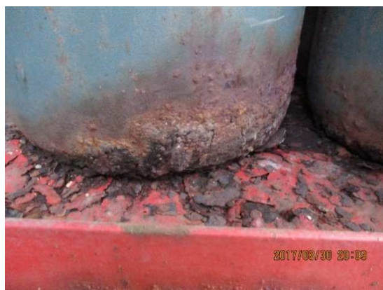
Figure 7.3-2 Photo of the Bottom of Corrosive Carbon Dioxide Fire Extinguisher Cylinder
