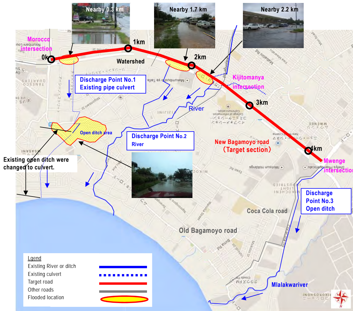
Figure 2-7 Drainage System around Existing Road
