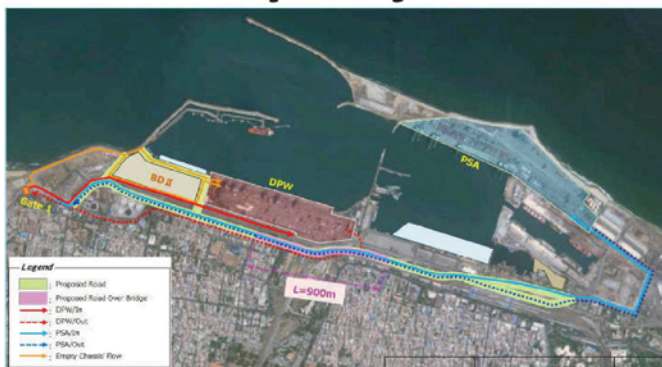
Traffic Flow Separation between DPW and PSA
