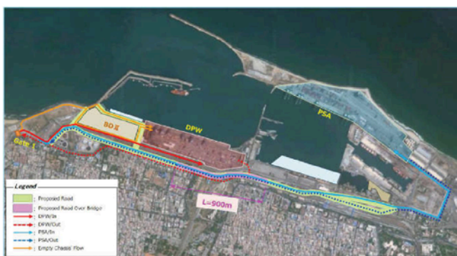
Traffic Flow Separation between DPW and PSA
