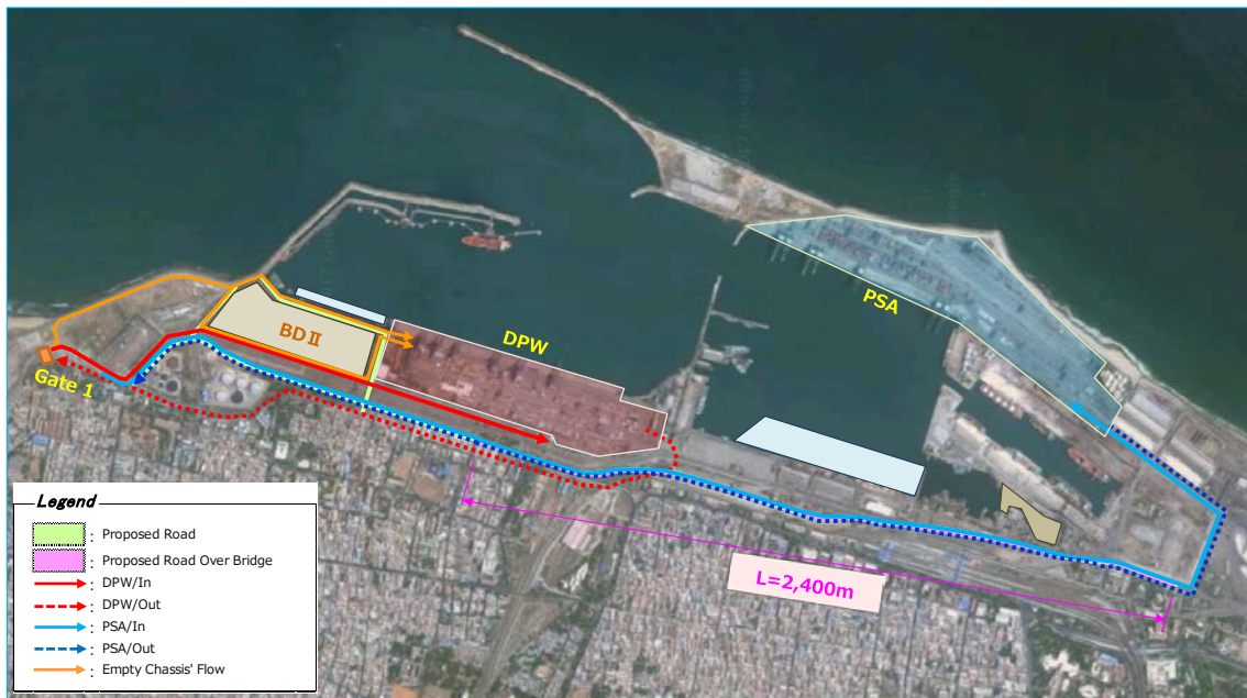
Figure 5-11 Traffic Flow Separation between DPW and PSA
