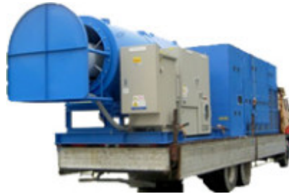
Picture 4 Example of Vacuum Device (Capacity 300m 3 /min)
