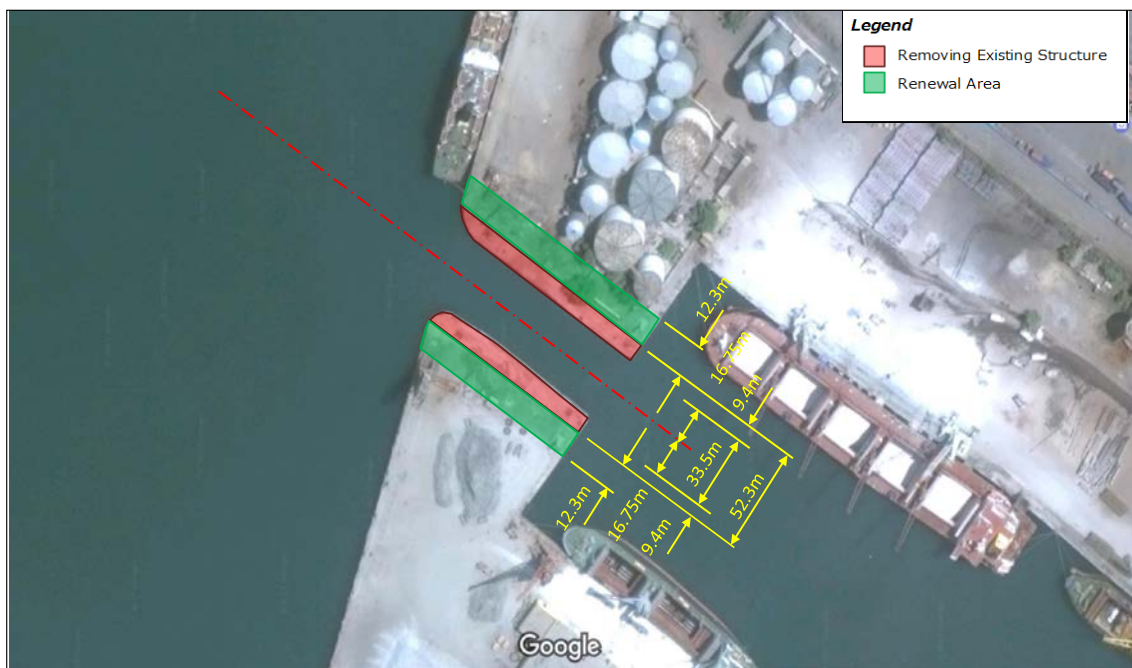
Figure 5-16 Widening of Jawahar Dock Entrance
