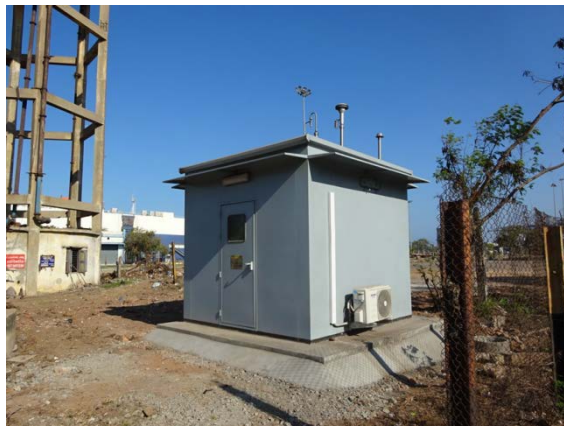
Picture 3-19 Air Quality Monitoring Station which will generate real time environmental data online
