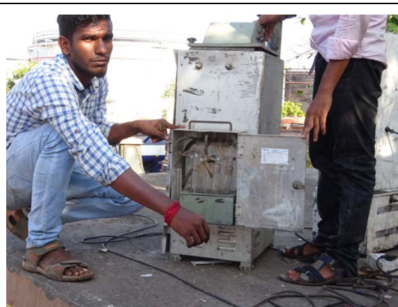
Picture 3-18 Air Quality Monitoring Instrument for NO 2 and SO 2 at Station A4 (Fire Office)
