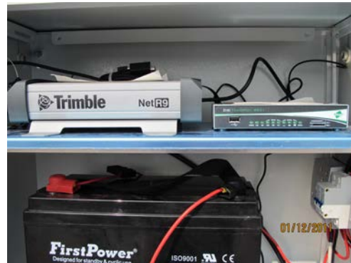
Photo 6.1.4 CORS (inside) (receiver, transmitter and battery)
