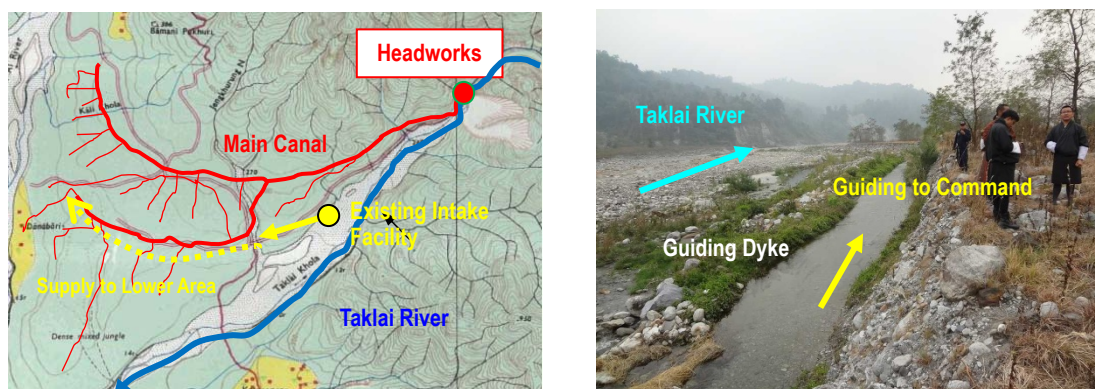
Figure 5.3.5 Situation of Intake through Existing Intake Facility
