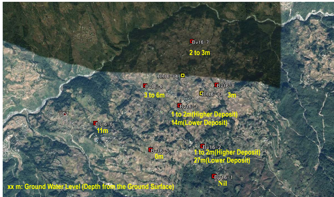
Figure 6.5.16 Location of Boring and Groundwater Level
