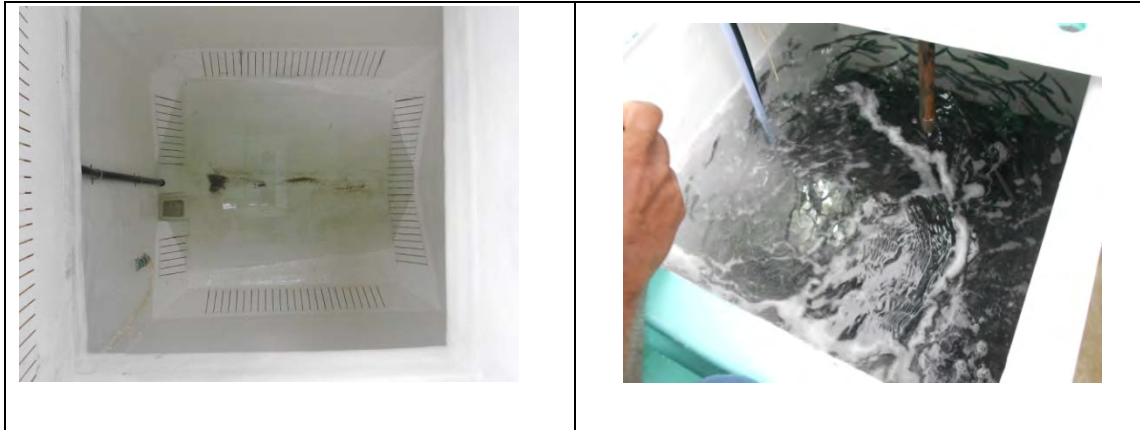
Figure-13 : Live bait tank of a Japanese fishing boat for skipjack pole-and-line
