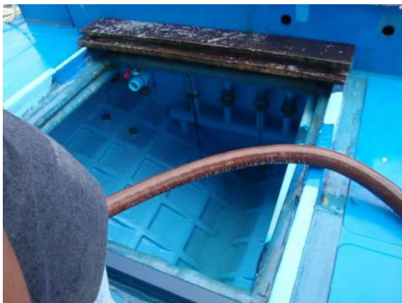
Live bait tank (before modification)
