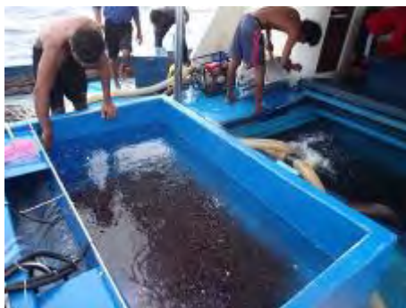
Fig. 1.2 Modified bait tank (at the center of the picture) and original tank (to the right)
