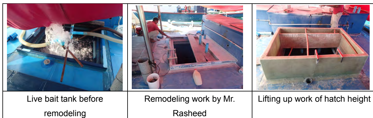
Figure 3: 1st live bait tank remodeling work
