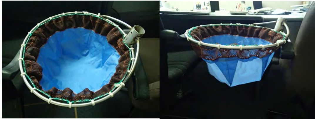
Figure 5: Modified scoop net with netting in the upper part and water proof material in below.
