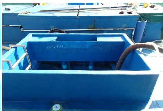
Live bait tank (after modification)
