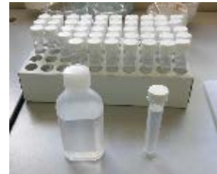
Fig.25 Sterile water for dilution (90 ml, 9 ml)
