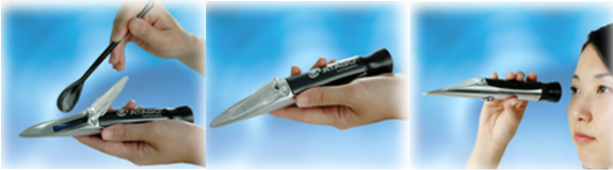
Fig.32 Measuring method of concentration of solution
