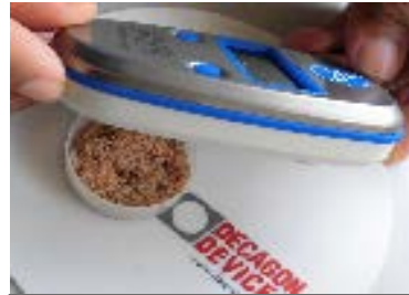
Fig.8 Set measuring cup with sample to the instrument
