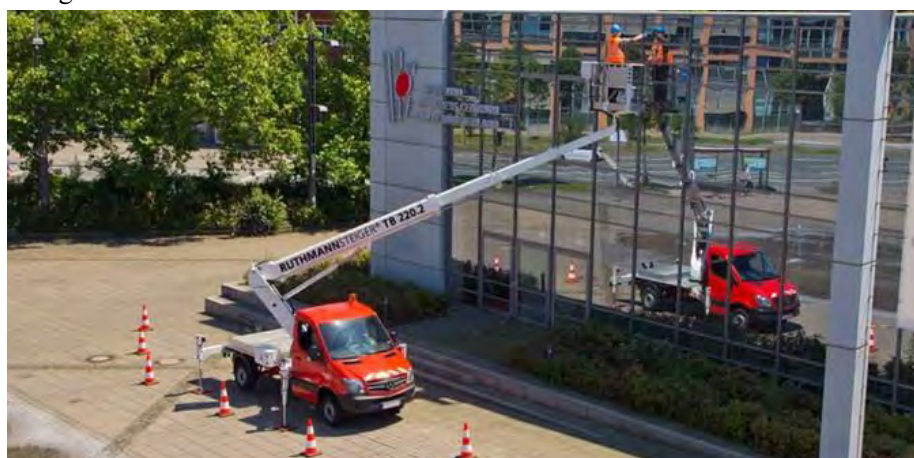
Figure 3-9 A bucket truck made in Europe
