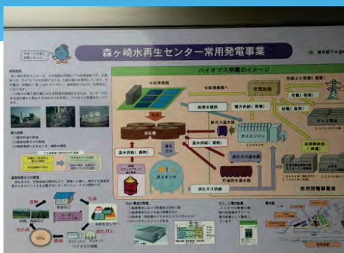
Diagram of using the sludge decomposition process to generate electricity
