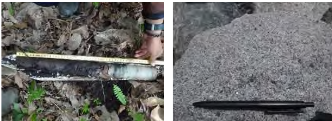
Figure 23 Field verification survey (Left: boundary with clay, right: basement granite)
