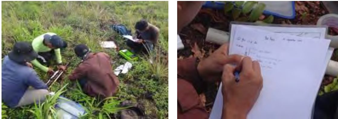
Figure 21 Field verification survey (left: coring, right: description of profile)
