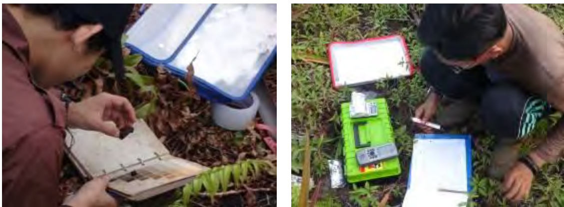
Figure 22 Field verification survey (Left: observation of color, Right: measuring bulk density)
