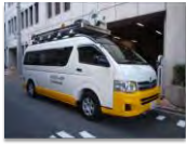
"Doctor Patrol" (Automatic Road Surface Inspection Vehicle)
