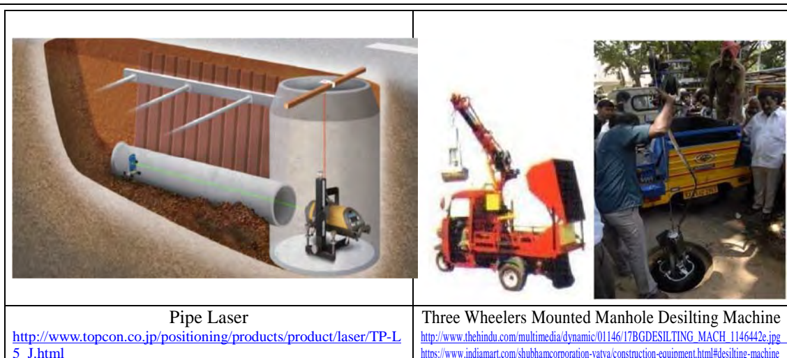
Figure 13.3.2 Images of Pipe Razer and Sewer Cleaning Car
